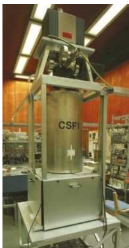
Figure 1.1 (a) International Prototype of the Kilogram, an accurate copy of the International Standard Kilogram kept at Sèvres, France, is housed under a double bell jar in a vault at the National Institute of Standards and Technology. (b) A cesium fountain atomic clock. The clock will neither gain nor lose a second in 20 million years.
